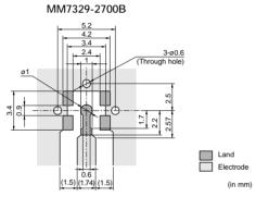
Pattern should be designed to match 50 ohm impedance circuit.
