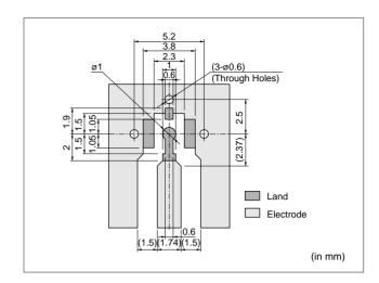
2. Standard solder stencil mask pattern Follow Standard solder stencil mask pattern to avoid the possibility of solder being trapped under connector.
