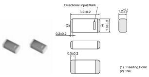
Terminal of "NC" should be connected to the floating land
