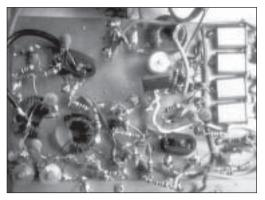
Shows only two coils in the RF filter, the third was added later. The upper coil is the VFO. The mixer transformer is seen on the lower right part of the picture.
