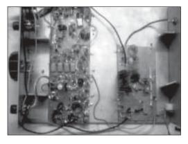
The big board has the entire exciter. The smaller board on the right is the linear
