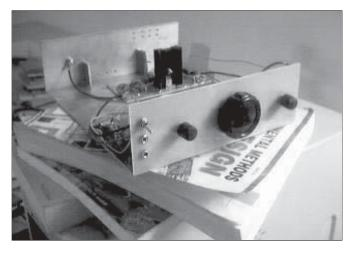
BITX is an easily assembled transceiver for the beginner with very clean performance. Using ordinary electronic components and improvising where specific components like toroids are not available, It has a minimm number of coils to be wourd. All alignment is non-critical and easily achieved exenvit but sophisticated equipment. The entire instructions to assemble the rig are given here along with relevant theory.
