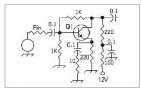
the collector to emitter is a multiple of the current flowing from the base to the emitter. Thus, if there is a small change in the current flowing into the base, there is a bigger change in the current flowing into the collector. What follows is a highly simplified explanation of working of the above amplifier.
