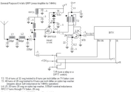
Use a clip-on heat sink for 2N2218, a small heat sink for IRFS10 with mic spacer
