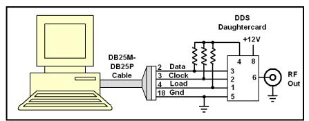
The Parallel port cable pin out. Note the pull-up resistors. Use about 2.2K.
