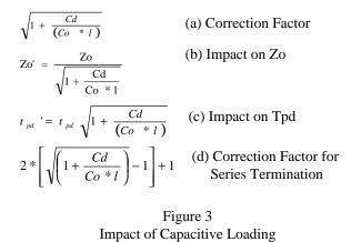
capacitive loads are charged through the series load, somewhat slowing down the rise time, and therefore the propagation time, of the trace. The adjusted correction factor for series termination is shown in Figure 3d. Note that in all these cases the adjustment factor collapses to 1.0 if Cd = 0.
