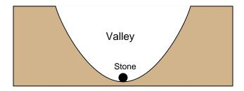
The stability of the stone in each of these scenarios represents the stability of a specific type of electrical feedback system. Which of these scenarios represents negative feedback, which represents positive feedback, and why?
