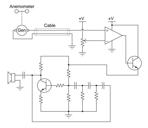
The circuit works well to warn of high wind speed, but when the wind speed is just near the threshold level, every little gust causes the alarm to briefly sound, then turn off again. What would be better is for the alarm to sound at a set wind speed, then stay on until the wind speed falls below a substantially lower threshold value (example: alarm at 60 km/h), reset at 50 km/h).
