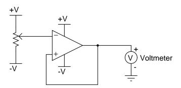
The output voltage will saturate at approximately +11 volts, or -11 volts, with the potentiometer having little or no effect.
