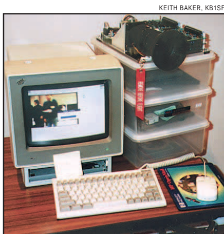
An engineering prototype of JAMSAT's SCOPE camera. The camera is above, and to the right, of the monitor. Phase 3D will carry two SCOPE cameras—wide angle and narrow angle. Both will provide spectacular color images.
