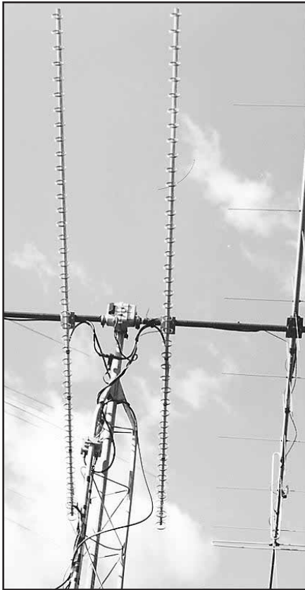
Twin 1.2-GHz loop Yagis are part of the ARRL Headquarters satellite station.
