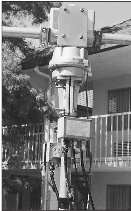
An az/el rotator moves your antennas from side to side (azimuth) and up and down (elevation).
