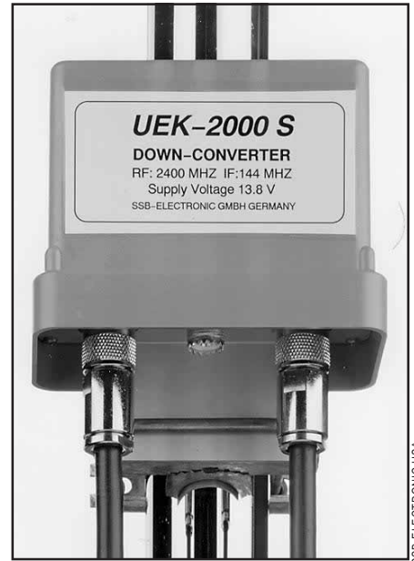
A 2.4-GHz receive converter typically converts the S-band signal to 2 meters. In some cases it is possible to purchase 2.4-GHz units that will convert all the way down to 10 meters. In either case, you must install the converter at the antenna.
