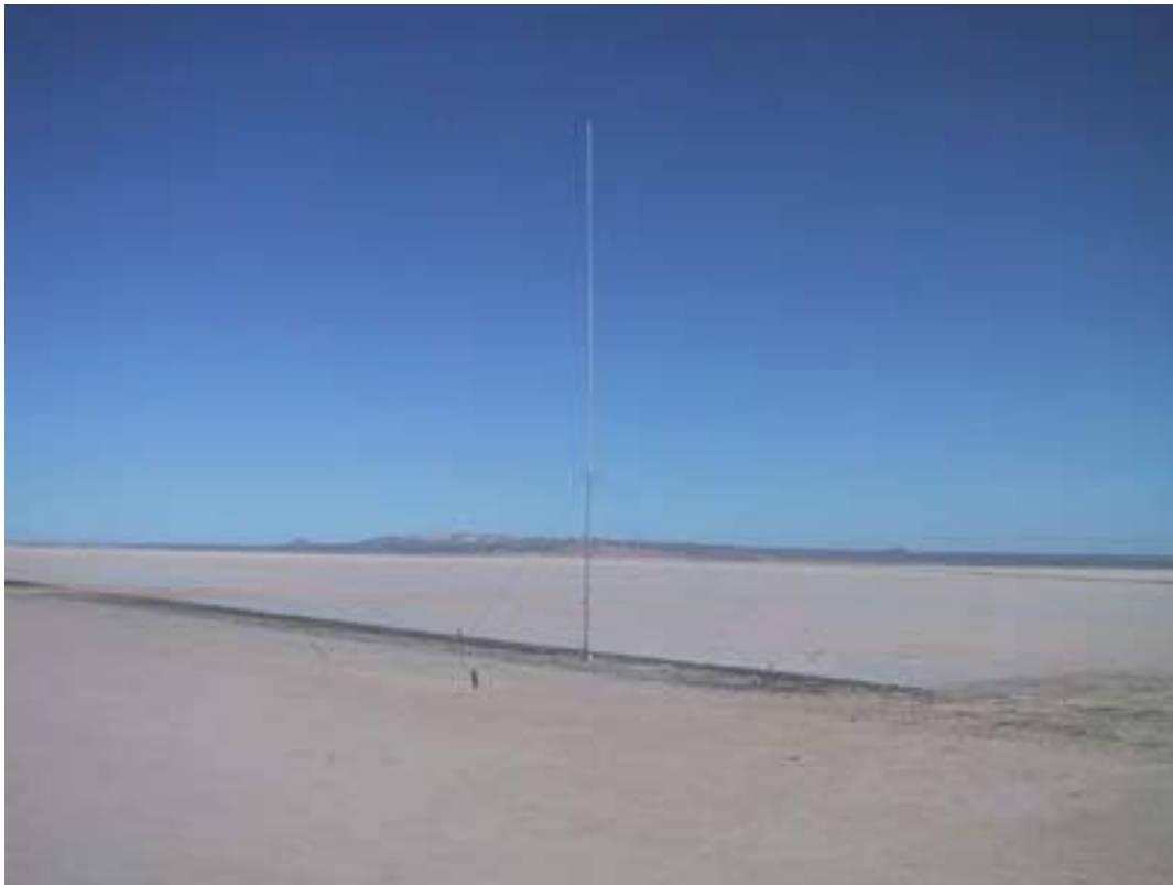
Figure 3. Installed Reference Quarter-Wavelength Reference Antenna
