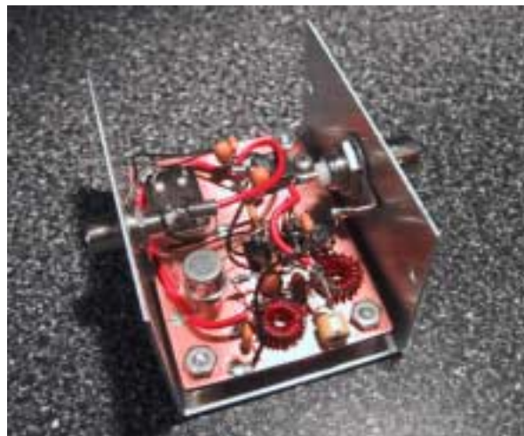
Figure 6. Custom Designed Low-Distortion Crystal Oscillator/RF Source
