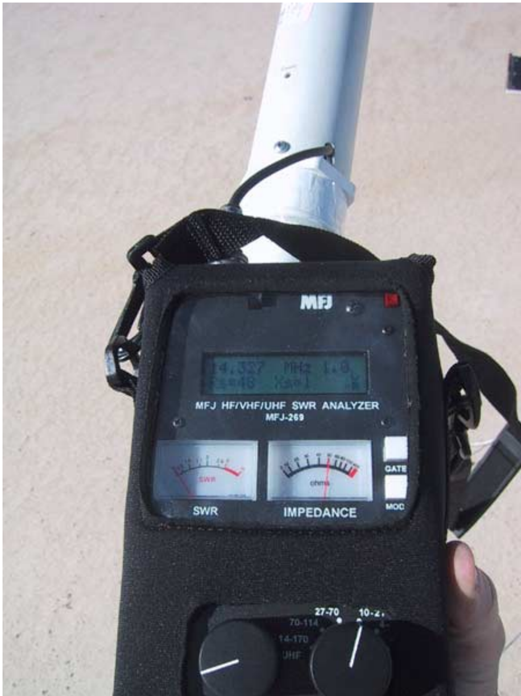
Figure 9. MFJ-269 Showing Excellent Source Match of Test Antenna During Test Antenna Setup
