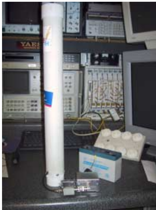
Figure 2b. Pre-installed “Backpacker” 20-Meter Test Antenna (Radome Installed)
