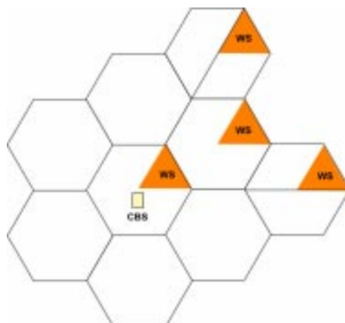
Figure 6.3 Multi-cellular deployment showing interfering regions
