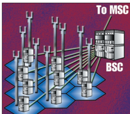
Figure 1. Conventional backhaul with one T1 span per base station. A backhaul with 9 cells means a $162,000/year T1 cost.
