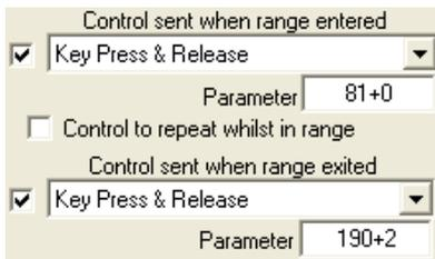
When my selected axis zone is entered, I am sending Key Press 81+0. Here the '81' is a KeyCode and '0' are the Shift keys I need. KeyCodes are listed in the Advanced User's guide—81 is 'Q'. The shift key combinations you can have are also listed in that document. Here I just want a plain Q (for FS's sound toggle—for which I should really have used an FS control of course), and I could use '8' or '0' for that.
