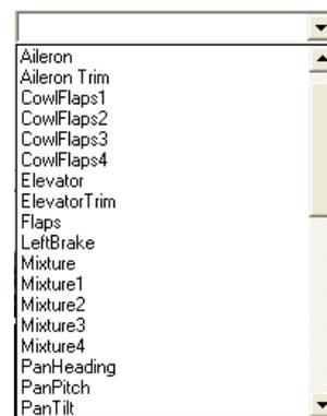
In the illustration you will see that you can assign up to four different controls to the one axis. You enable each of the four by checking it to the left. This provides full flexibility for "mapping" your levers to selected engines and so on. Together with the aircraft specific option and the automatic loading of the correct settings (and calibrations, if you calibrate in FSUIPC), you have the utmost
