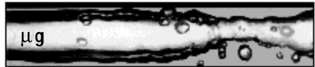
Side views of water and air flowing through a clear pipe. At 1g, the air stays on top. In microgravity, the air can form a core down the center of the pipe.
