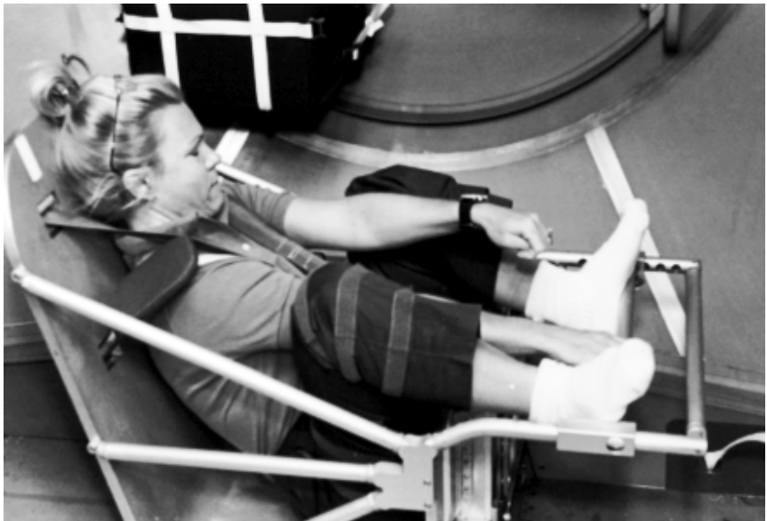
Payload Commander Dr. Rhea Seddon is shown using the Body Mass Measurement Device during the Spacelab Life Sciences 2 mission. The device uses the property of inertia to determine mass.
